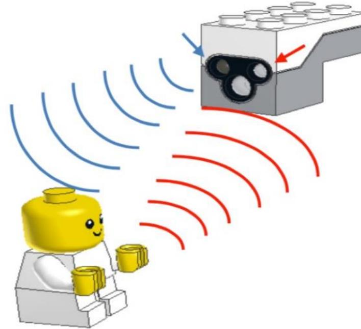
Figure 37: Sending/Receiving an infrared signal
