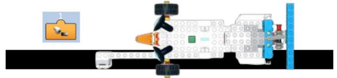
Figure 52: Follow the line - Take 2 measurements on the black line
