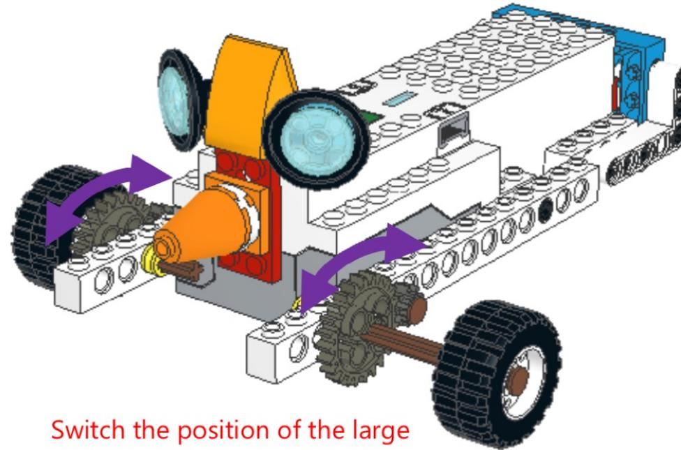
Switch the position of the large Gear with the small Gear
